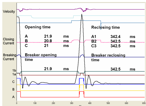
Figure 3.2a O-0.3s-C test without both sides grounded
