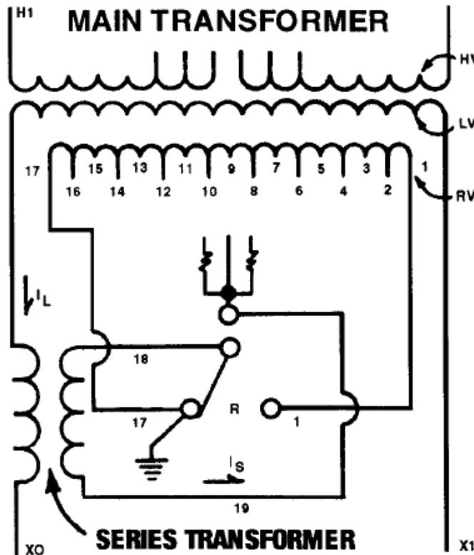
Fig. 1: Schematic of a tap changer with a series transformer
