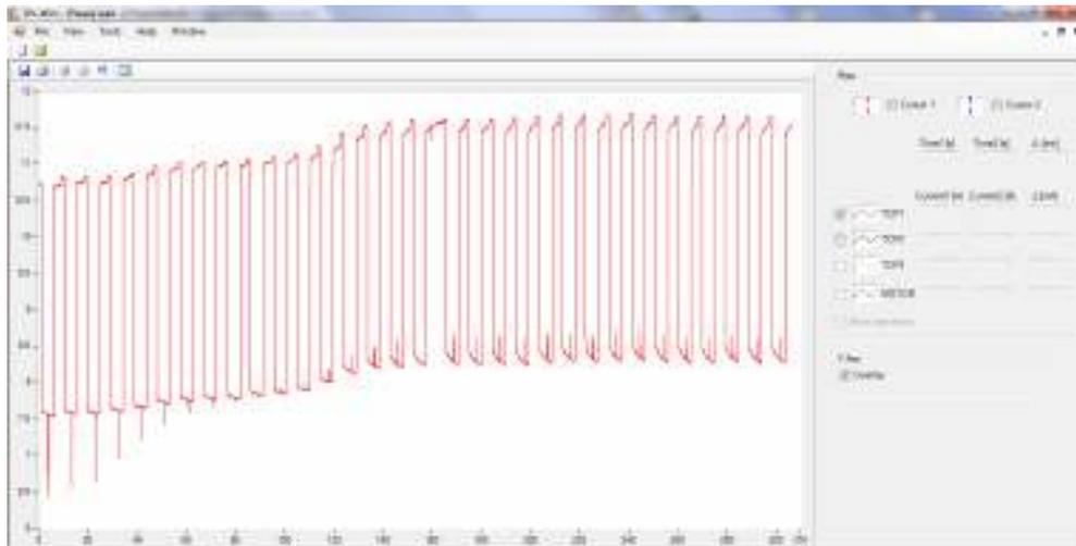
Fig. 4: Complete DRM graph of phase X1-X0 with series transformer
