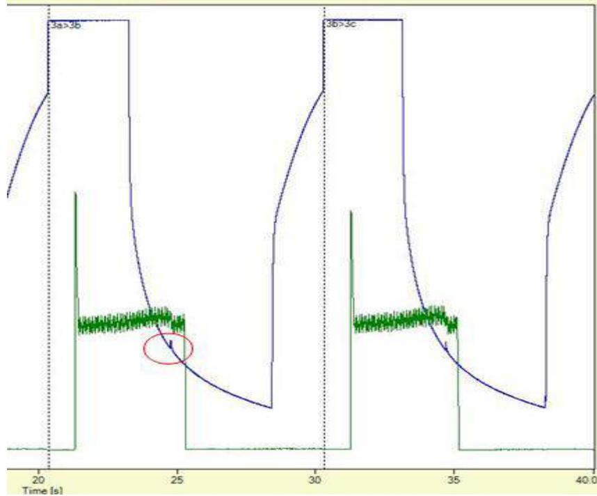
Fig. 2: Series transformer DVtest graph, a transition is marked with the red circle, motor current is green
