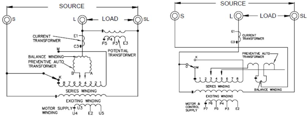
Figure 1. Schematic of two single phase regulators type A (left) and type B
