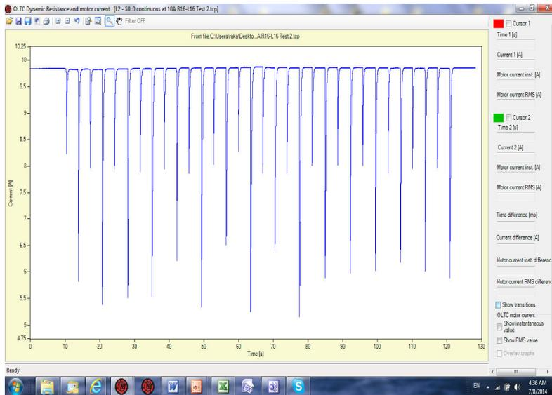
Fig 6. DVtest graph using SL to L connection with normal ripples
