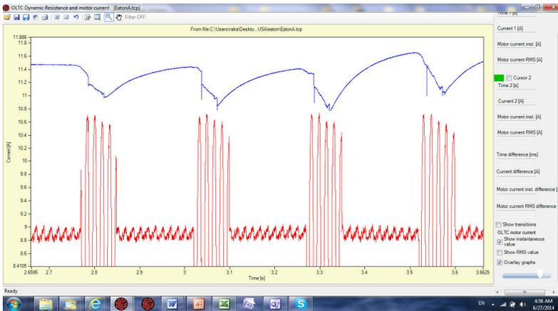
Figure 3. Four transitions in one second of a fast regulator
