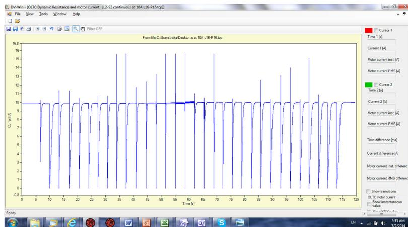
Fig.5. DVtest graph using S to L connection showing very high ripple
